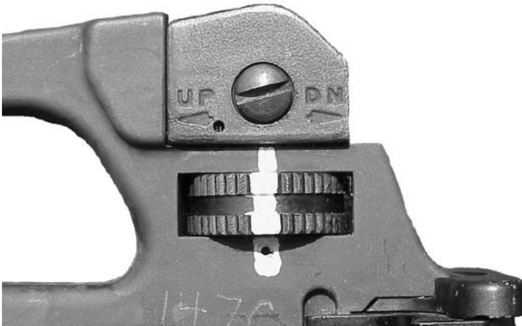
Figure 5-6 Rear sight initial setting
