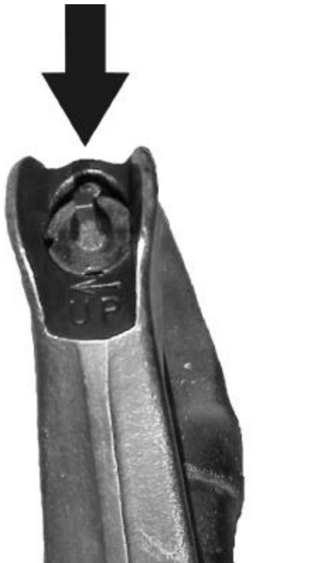
Figure 5-4 Front sight detent
